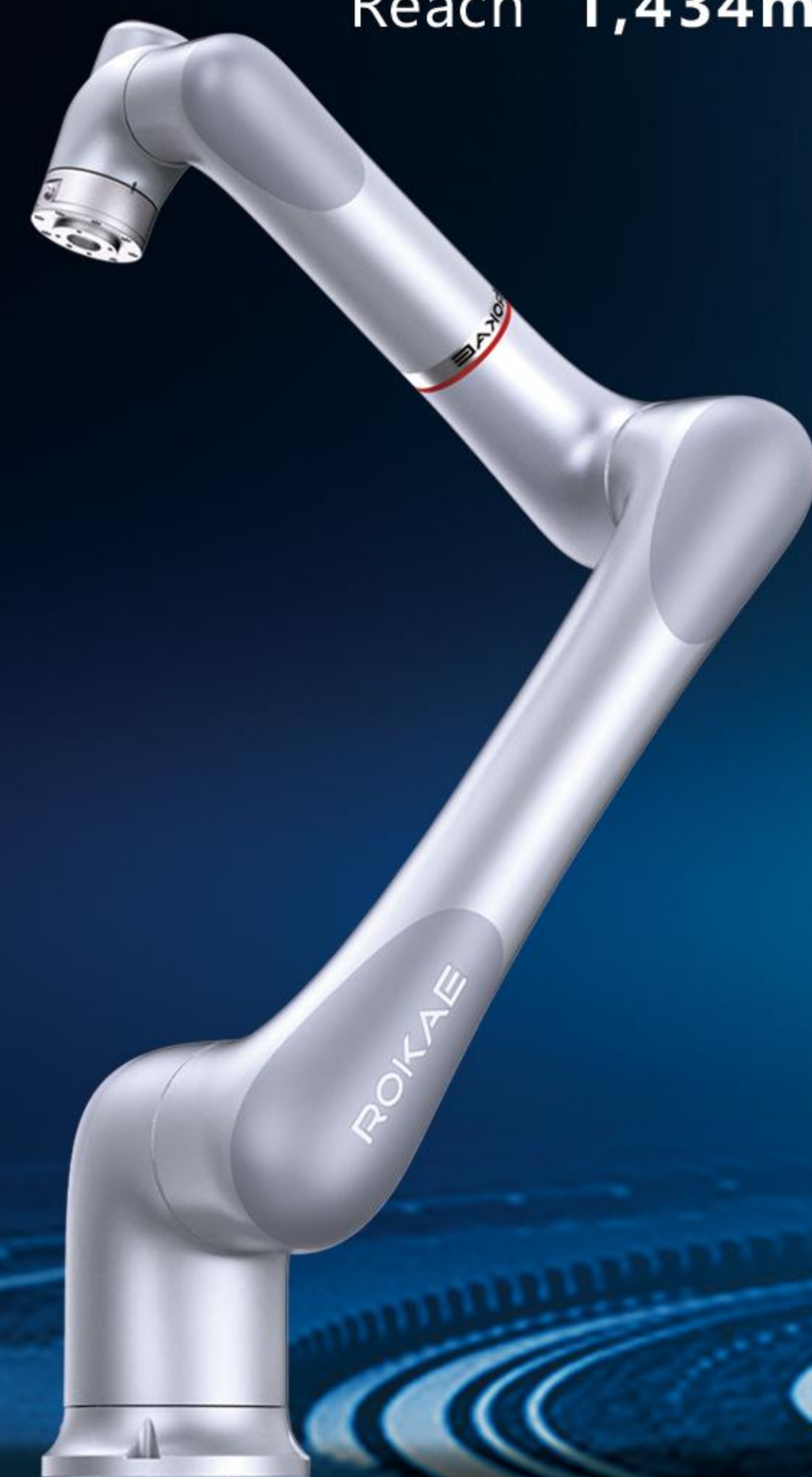
Model CR12-C Payload 12kg Reach 1,434mm
