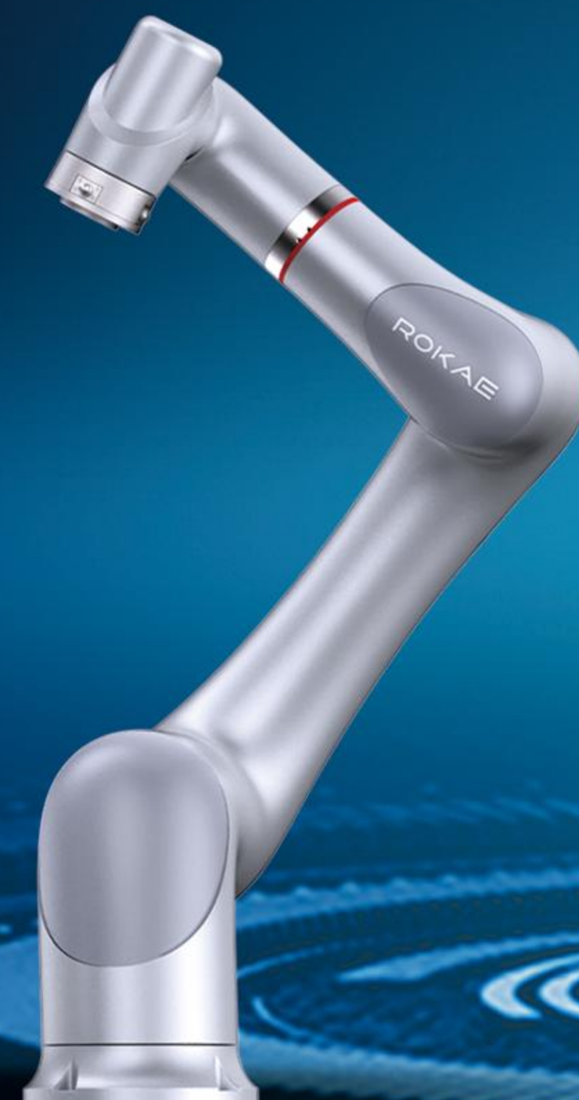
Model CR18-C Payload 18kg Reach 1,062mm
